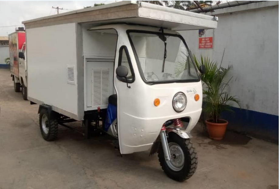
Tricycle mounted with refrigerated container with solar panels, Li-ion battery & pay load of 400 kgs
