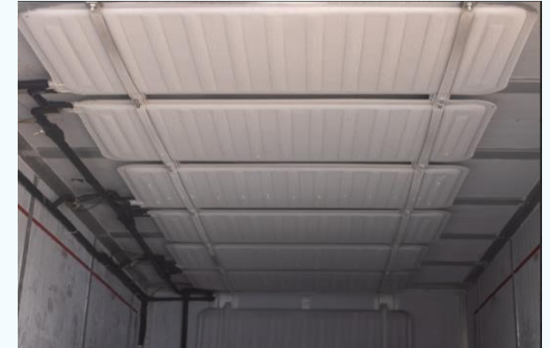
PCM plates mounted on a transportation truck for medium haul
